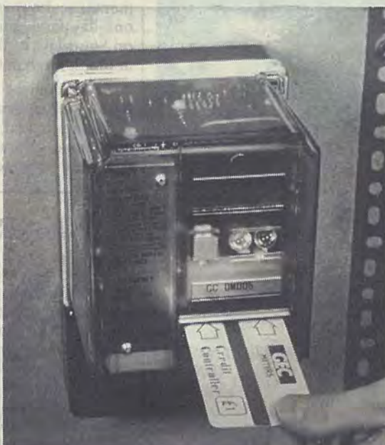
Below, an experimental meter which uses plastic credit cards bought in advance, to purchase pre-determined amounts of electricity
